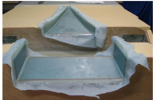
*Figure 3 – Peelply applied to Cosy Aircraft components*
