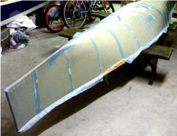
*Figure 1 – Prototype Canoe with Peelply applied*
