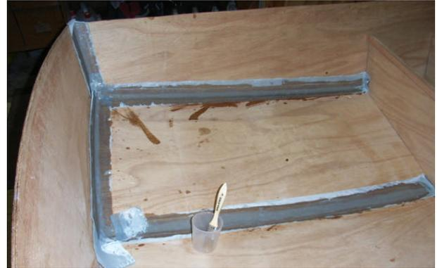
*Figure 2 – Stitch N Glue joints with Peelply applied*
