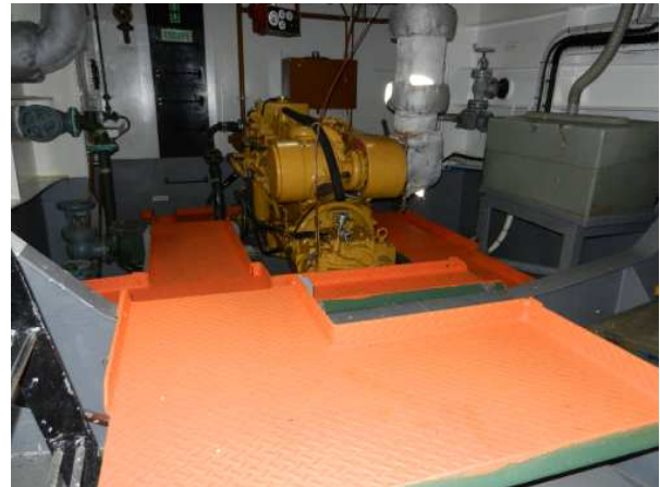
Figure 4 – Machinery Space Deckplates TREDGRIPPED
